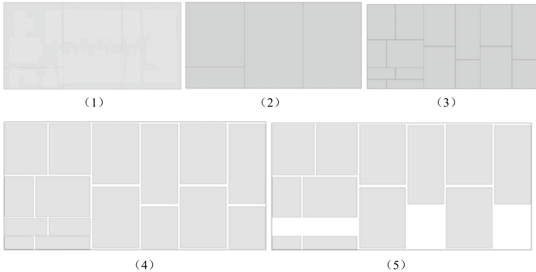
Fig. 35.5 Diagram of plot generation (1) Zoning based on original substrate (2) Zoning (3) Texture subdivision (4) Plot setback (5) Plot screening
