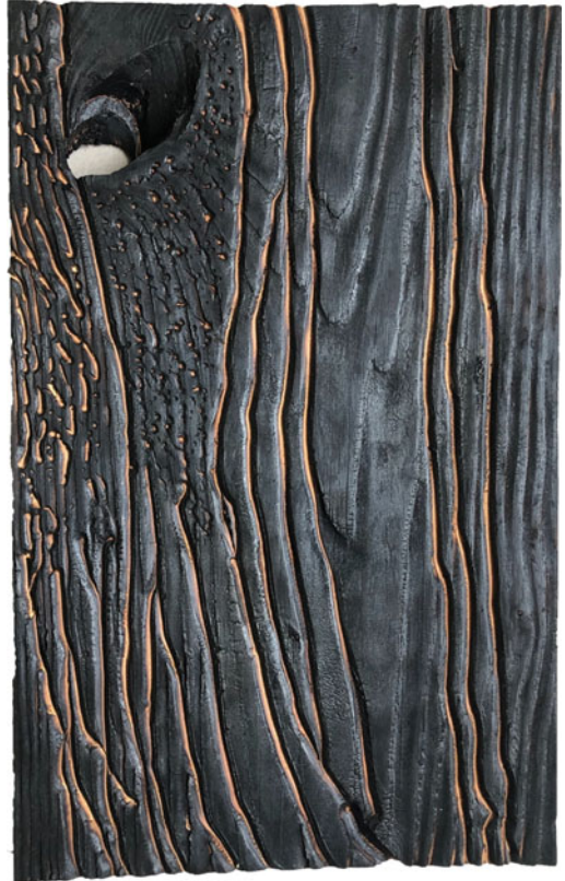
Fig. 12.25 A material treatment experiment using a torching technique referred to as Shou Sugi Ban creates tactile effect. Image ©
