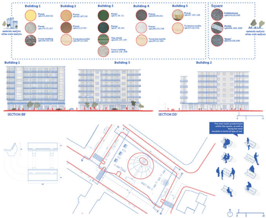
Fig. 10. 2D representation with metric, material and colorimetric data. Editing arch. G. Santoro
