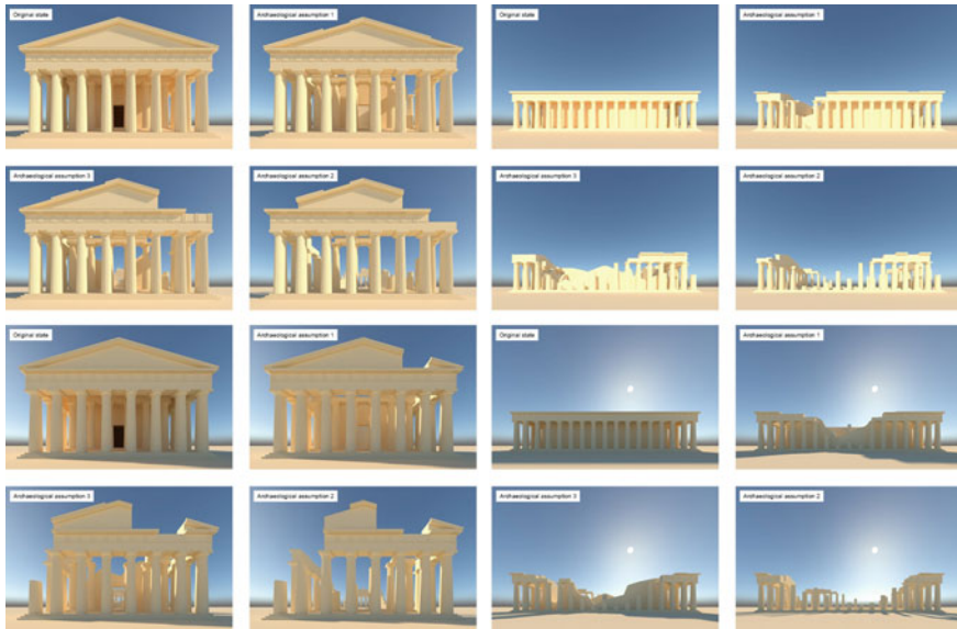
Fig. 2 States of destruction of one of the synthetic models representing an octastyle Greek peripteral temple. From the original state, the 3 states of ruin of the four facades of the building are shown. Modelling and rendering E. Delgado-Martos
