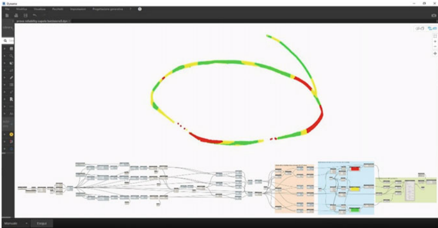
Fig. 8 Evaluation of the deviation on the dome’s generatrix and directrix (Editing A. Tata, P. Maiezza and S. Brusaporci)
