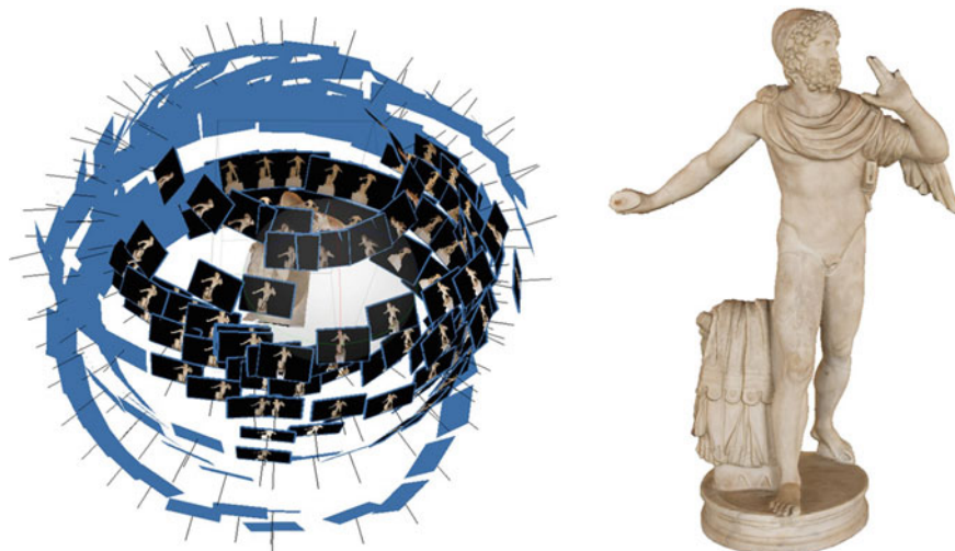
Fig. 3 Ulysses statue, photos alignment and construction of the dense point cloud. Elaboration in Agisoft Metashape Professional, version 1.6.1 (Modelling and rendering: M. Ciammaichella and G. Liva)
