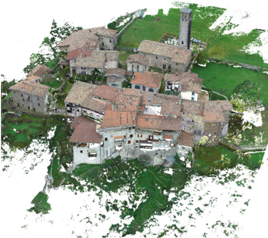
Fig. 2 The complete point cloud of Cornelio dei Tasso produced by combining laser scanning and photogrammetric point cloud. Modelling F. Fassi
