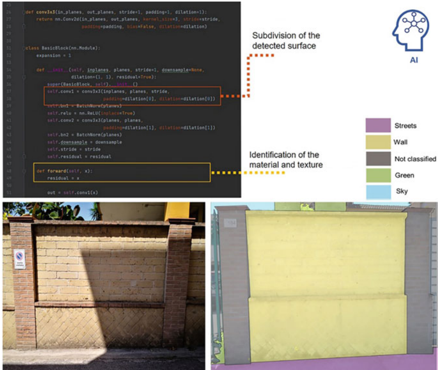
Fig. 9 Employment of a neural network for the individuation of construction elements in the image (Editing: G. Antuono)
