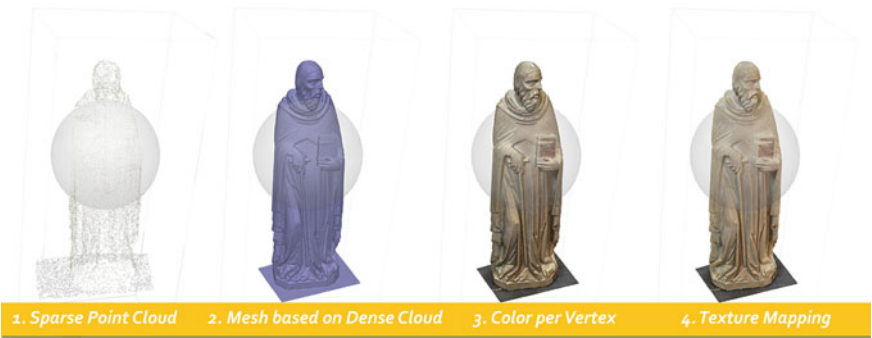
Fig. 4 Digital Photogrammetry using Metashape software. The steps in the automatic 3D modeling process (Image: G. Attademo)
