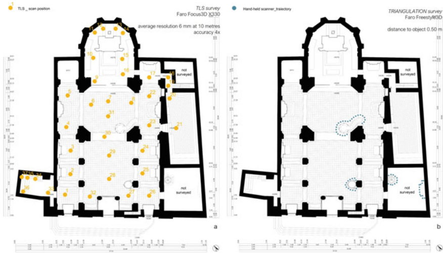
Fig. 2 Data acquisition schemes with TLS (a) and hand-held scanners (b). Image V. Cera, A. Origlia
