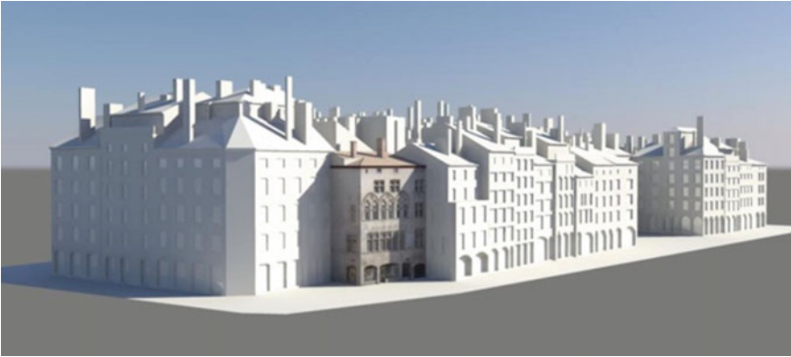
Fig. 4 Parametric design of the buildings of the Vieux Lyon district, France (untextured). The Maison du Chamarié (textured), because of an excessive amount of descriptive parameters, had to be designed manually (3D modelling and rendering: R. Saleri 2008–2009)
