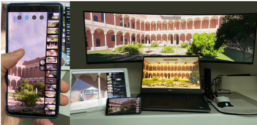
Fig. 12 The WebVR project of the Baths courtyard is navigable via the web and multiple devices such as VR headsets, mobile phones and tablets (Source F. Banfi, D. Oreni)
