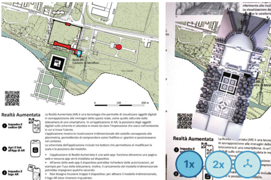
Fig. 9 Left: detail of the physical panel, showing the map of the area, the AR target, a QR code to access the web app, and a guide for the user (bottom). Right: screenshot of the web app showing the AR function and the buttons to activate different visualisation modes (Editing: V. Palma)
