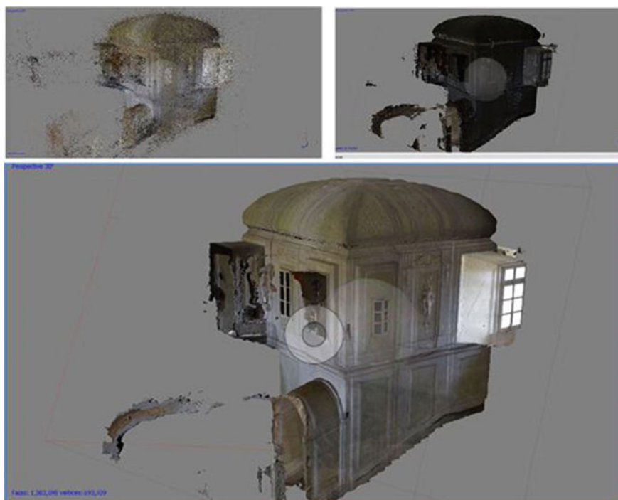
Fig. 3 Photogrammetric survey of the Monumental Staircase. a Point cloud. b Dense cloud. c Textured mesh. Modelling A.L. Pecora
