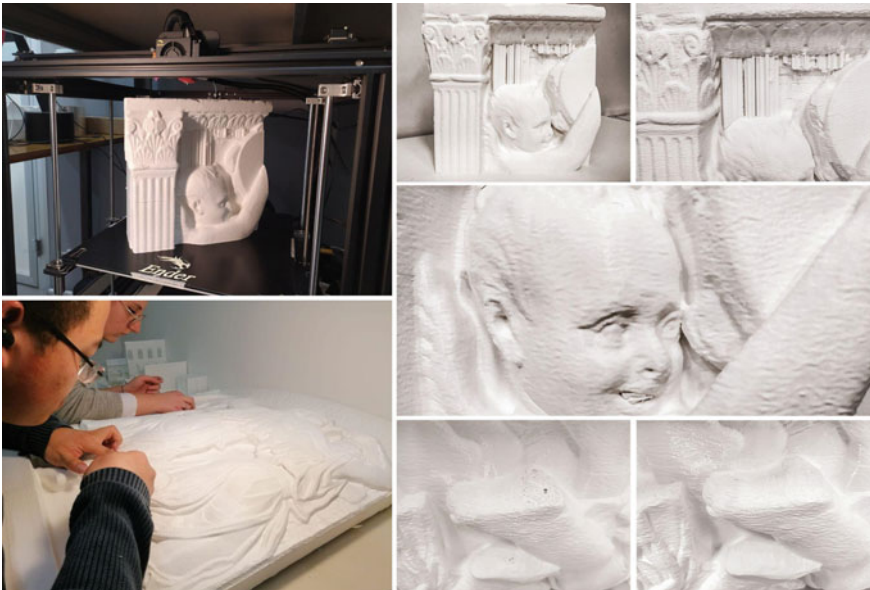
Fig. 8 The 3D printing process and the removal of any imperfection from the printed surface (Photos: F. Picchio)
