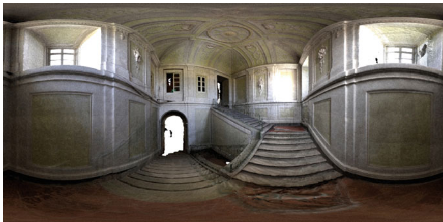
Fig. 12 A panoramic image, developed flat, of the virtual environment obtained from photogrammetric surveys. Modelling A.L. Pecora
