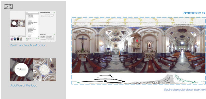
Fig. 11 Post-processing of equirectangular produced by laser scanner. Editing authors
