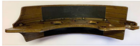
Fig. 11 Industrial brake shoe attached with shims investigated in [9]
