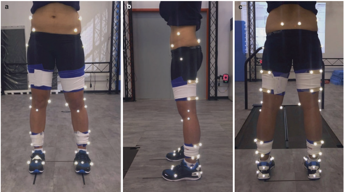
Fig. 4 (a–c) The reflective markers used during kinetic data capturing [Reproduced from [26] (License: Creative Commons Attribution License)]
