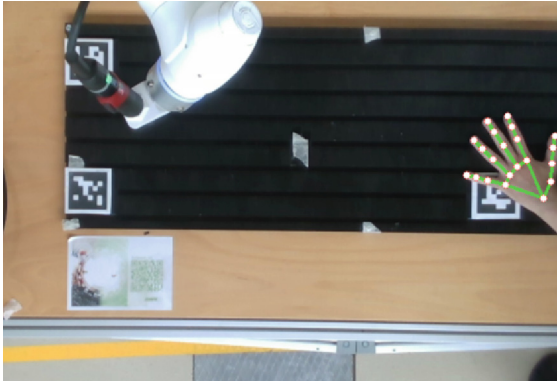
Fig. 9. Hand detection algorithm using OpenCV.
