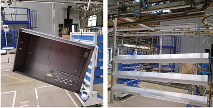
Fig. 5. Products hanging on a traverse [4]
