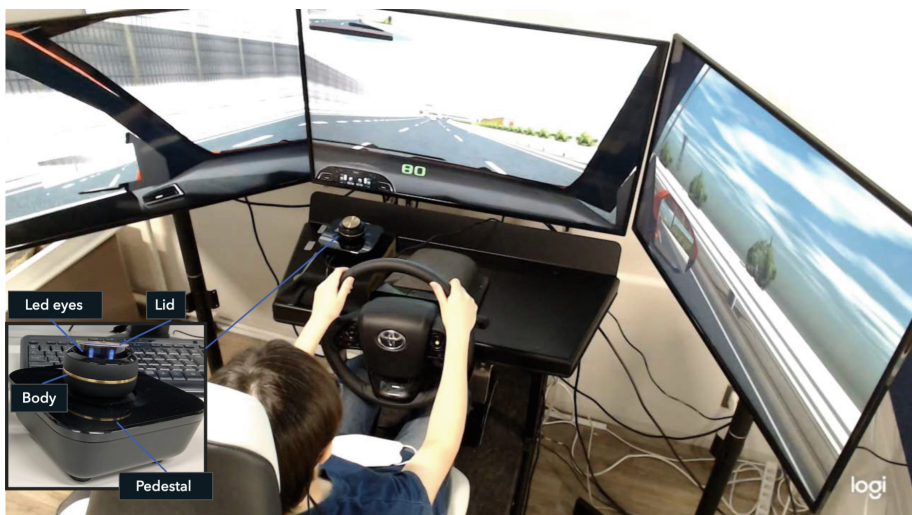
Fig. 1. Robotic human-machine interface (RHMI) prototype consisted of a lid, body and pedestal. Its LED eyes are shown under the lid. The figure also shows the experimental environment. The RHMI was oriented from participants toward the driving environment.
