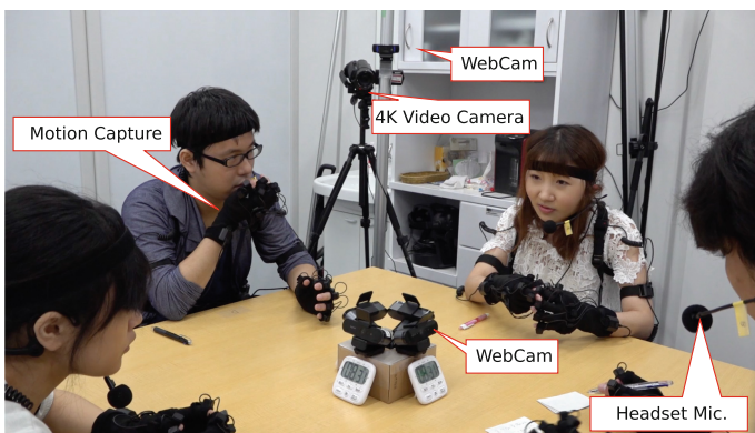
Fig. 1. Setup of the data corpus recording experiment. The female participant who is facing the camera is the L2 speaker who is perceived highest level of Japanese proficiency (H1)
