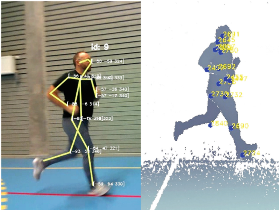
Fig. 4. Examples of skeleton tracking from the drone and its Intel RealSense L515 camera using two different skeleton tracking software solutions. The left part shows Cubemos Skeleton Tracker SDK [8] and the right part shows NuiTrack [1] overlaid on the depth data. The two examples show the same subject, but different experiments.
