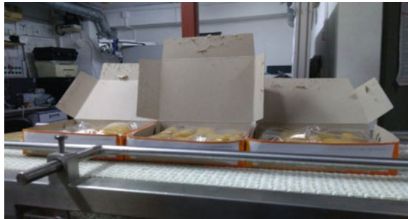
Fig. 5 The result of the algorithm. The nuggets do not protrude over the edges with the box
