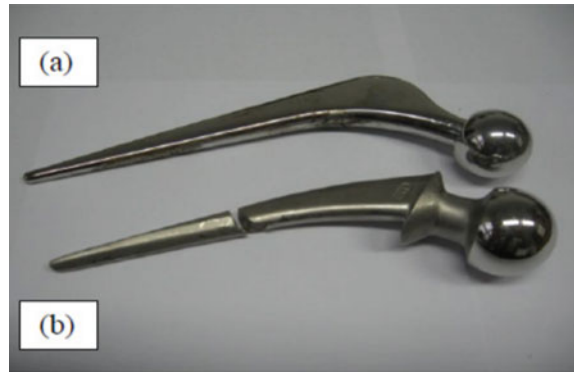
Fig. 1.11 Failure of stainless steel implants in human body: a corrosion on surface; b mechanical fatigue (reprinted with the kind permission of Biomedical Journal of Scientific & Technical Research, [33])
