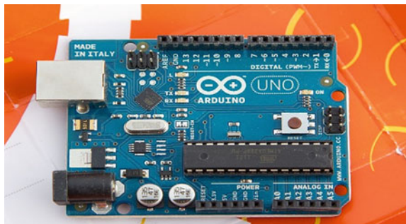
Fig. 2 Platform of Arduino type UNO
