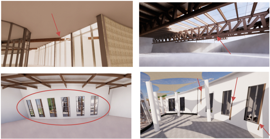
Fig. 9. Examples of the building systems integration errors as disclosed via VR technique.
