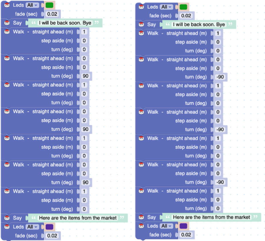
Fig. 3. The example of incorrect (on the left) and corrected (on the right) code for Task 2.
