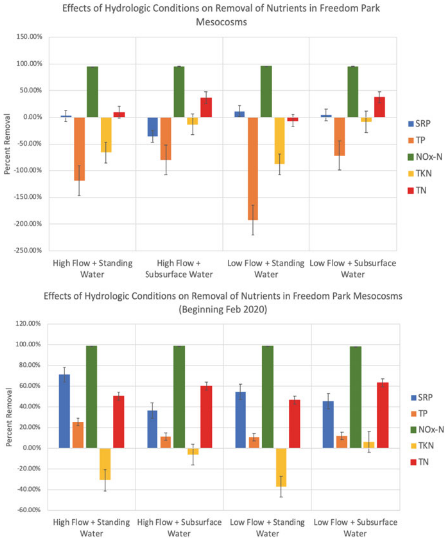
Fig. 15.5 Average removal efficiency \pm standard error for each nutrient species for four separate hydrologic conditions for Freedom Park mesocosms for (a) full 2.5-year study and (b) final year Feb 2020 to Feb 2021. The bottom chart excludes data before February 2020 to illustrate the significant improvement in nutrient retention in the last year of the study
