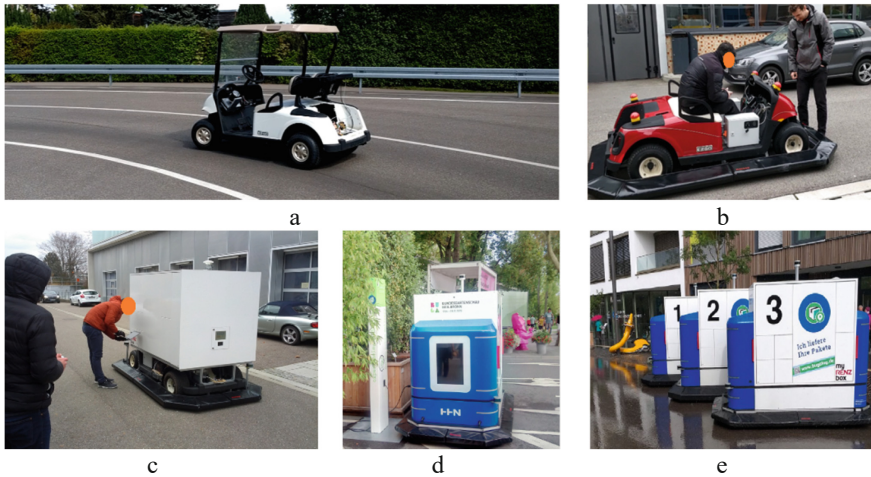
Fig. 9. Vehicle development cycle: (a) chosen vehicle; (b) bumper integration; (c) parcel box integration; (d) final vehicle at charging station; (e) vehicle fleet.
