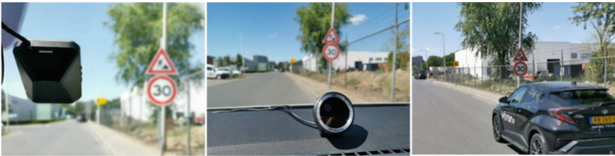
Fig. 1. The V-tron ISA system was used in the study presented in this paper. It consists of a camera (right) that can recognize the speed sign on the road, a round-shape display (middle) that can show the current speed limit, and other safety-related information.
