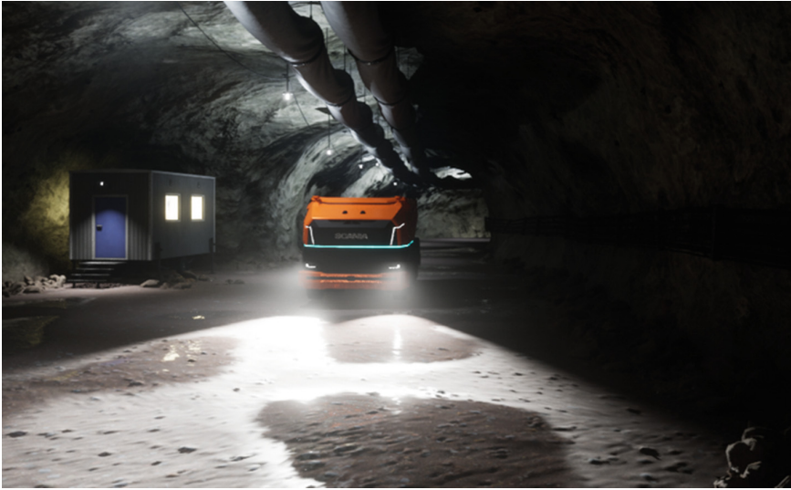
Fig. 1. A The cabless automated vehicle with eHMI to signal vehicle’s intentions in the underground mine simulation.
