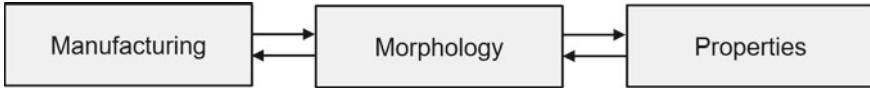
Fig. 1 Scheme of Manufacturing–Morphology–Property Relationships (MMPs) for mechanical components as they are studied in the present book. The arrows indicate the relations, which lead either from the manufacturing to the properties or in the reverse direction, from desired properties to a suitable manufacturing process
