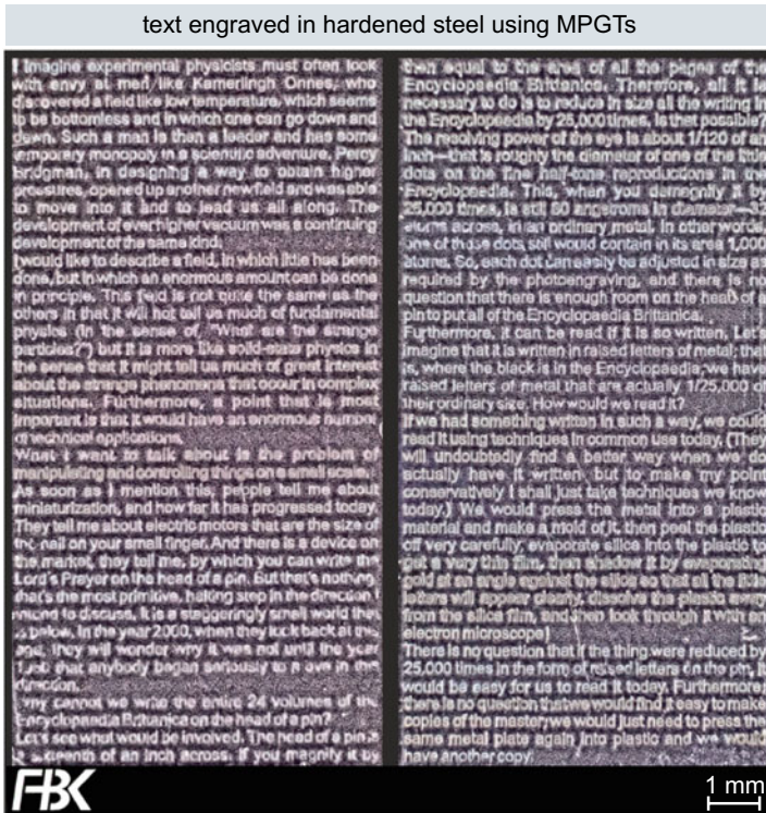
Fig. 27 Text engraved in a workpiece made of 16MnCr5 using six MPGTs in a micro grinding process according to [33]
