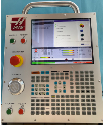
(a) A Haas controller simulator.
