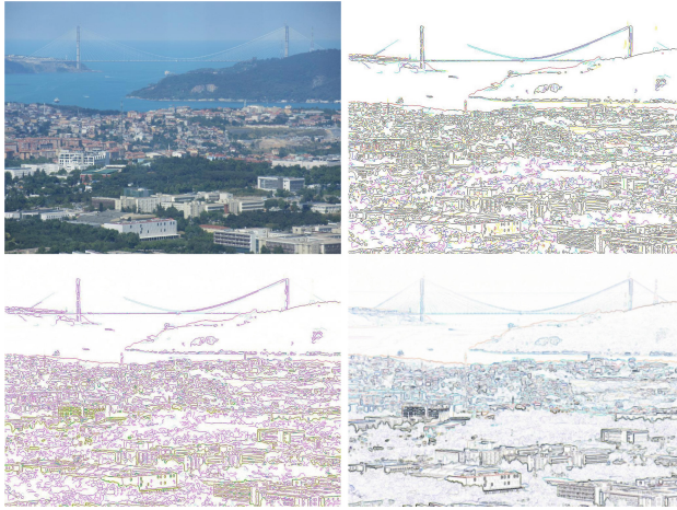
Fig. 1. Skyline of Istanbul and Bosphorus Bridge at RGB Scale (Source, Canny; ACO, Gabor)
