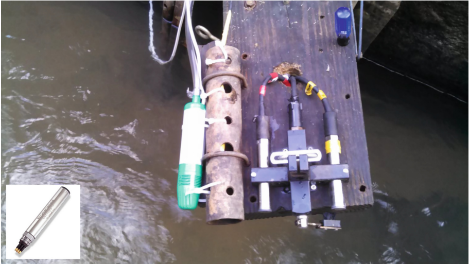
Fig. 1. Turbidity/fDOM sensor mounted on a board immersed in the water. The image in the corner is a Turner Designs Cyclops-7 submersible sensor.
