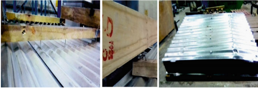
Fig. 6 Nails removal and metal sheets deformation under the effect of applied uplift forces
