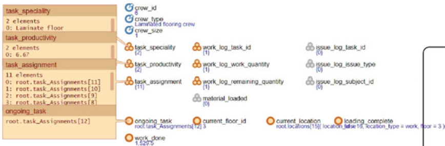
Fig. 10 Agent instance of a crew generated from input data
