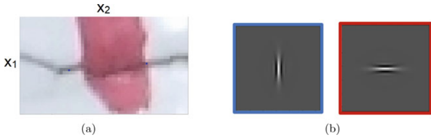
Fig. 4 a Input image with chosen endpoints; b Real part of the cake wavelets with angle \theta equal to 0 and \frac{\pi}{2} respectively.
