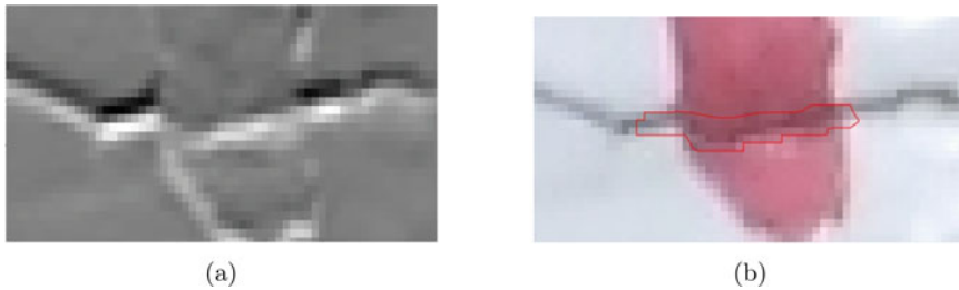
Fig. 7 a Oriented edge filter applied to the image shown in the Fig. 4a; b Crack edges detected with the ET method.
