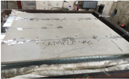
Fig. 7 a, b The fitting of the samples onto the furnace opening
