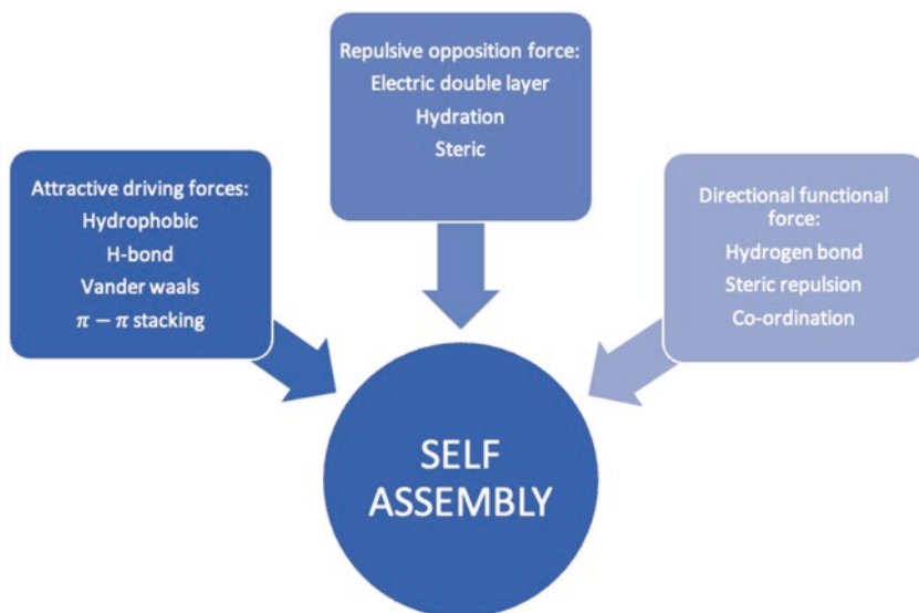
Fig. 6.1 The forces acting in the process of molecular self-assembly
