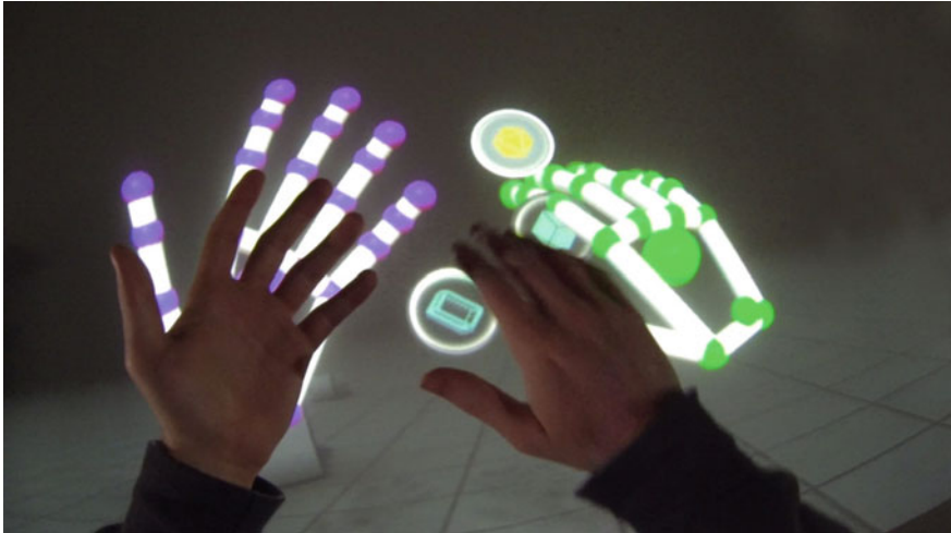
Fig. 5 Ultraleap’s no touch interface with advanced hand-tracking
