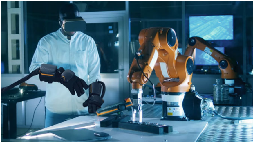
Fig. 13 Haptx gloves with haptic feedback
