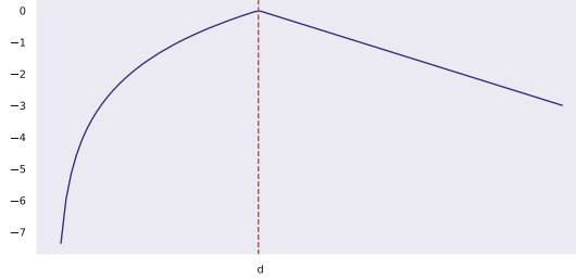
Fig. 7. Cohesion-Collision reward function: the red vertical line represents the target distance d . The portion of the graph to the right of the red line represents the influence of the cohesion term, while the left one represents the influence of the collision term. (Color figure online)
