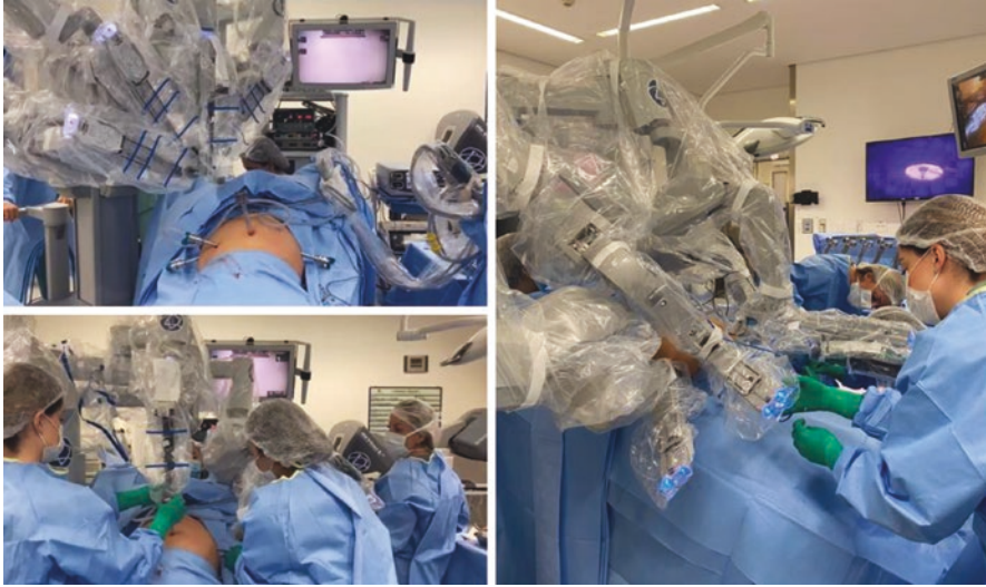
Fig. 6 Side docking for the lower abdomen and pelvis in the Si platform. (Photo: courtesy of Dr. Renato Moretti-Marques's personal archive)
