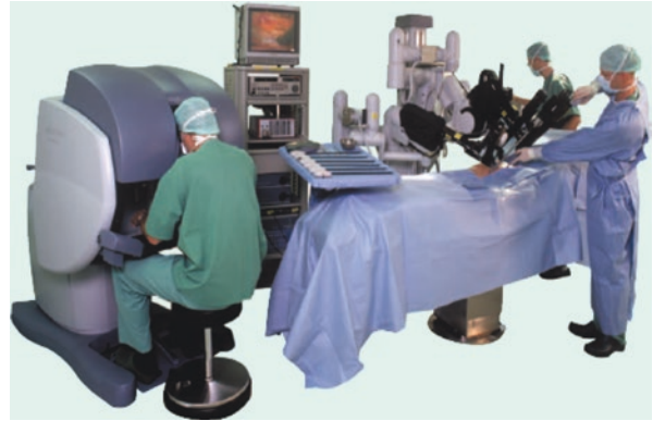
Fig. 7.1 The da Vinci surgical system consists of a master console and teleoperated patient-side robot (Okamura et al. 2010)
