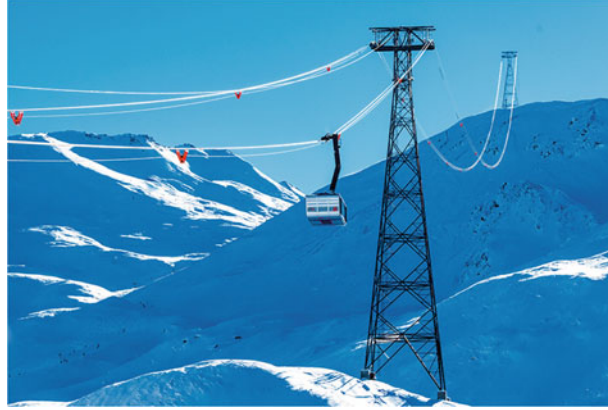
Fig. 17.1 A picture of aerial tramway: mobile and fixed cables, vehicle, and tower (photo: Doppelmayr website)
