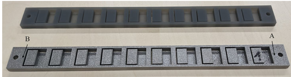
Fig. 21.1 Metamaterial beams made of different types of base material
