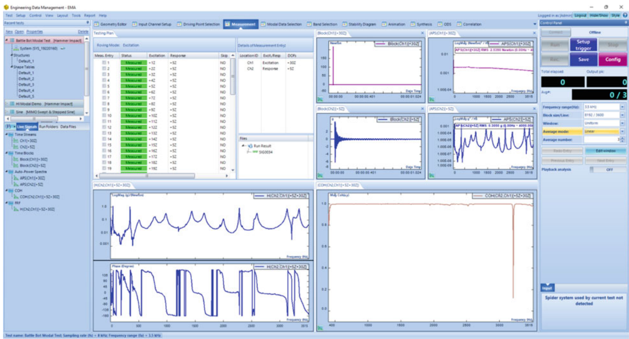
Fig. 1.4 Hammer impact measurement of the robot
