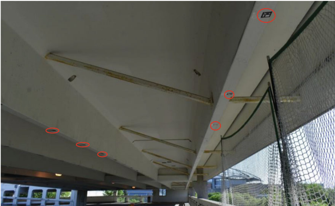
Fig. 18.3 Outdoor experiment setting with fiducial markers attached to the ceiling for UAV localization
