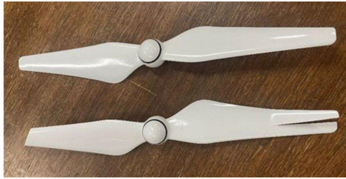
Fig. 15.2 DJI OEM 9450S Quick-Release Propellers, the upper is an undamaged prop and the lower is a damaged prop; broken tip on the left and split tip on the right
