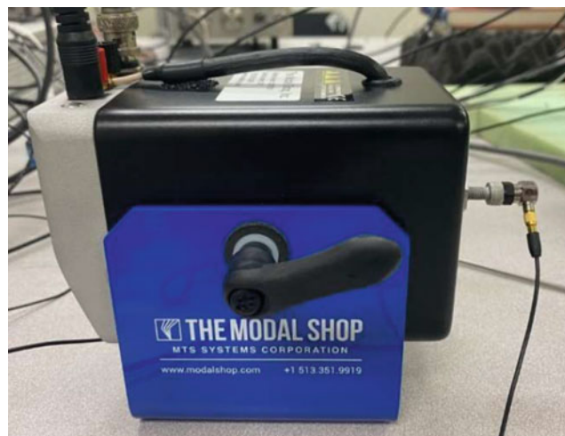
Fig. 12.4 Setup used in shaker characterization tests
