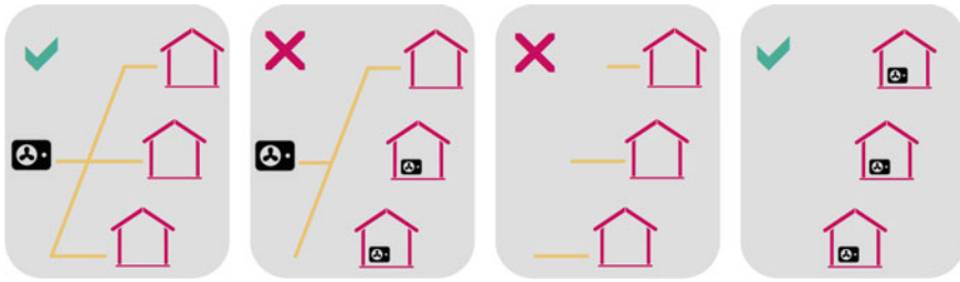
Fig. 2 Building owners technology choices and local infrastructure should align for an effective and cost-efficient operation: local or district heating with a high proportion of connected buildings, or individual heat supply solutions without investments in common infrastructure
