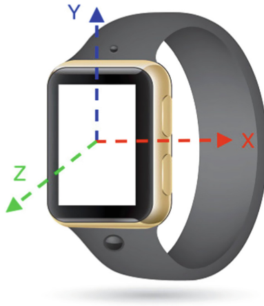
Fig. 2. Visualization of the three axes of the acceleration sensor of a smartwatch. Source: Cole et al., 2017 [10]
