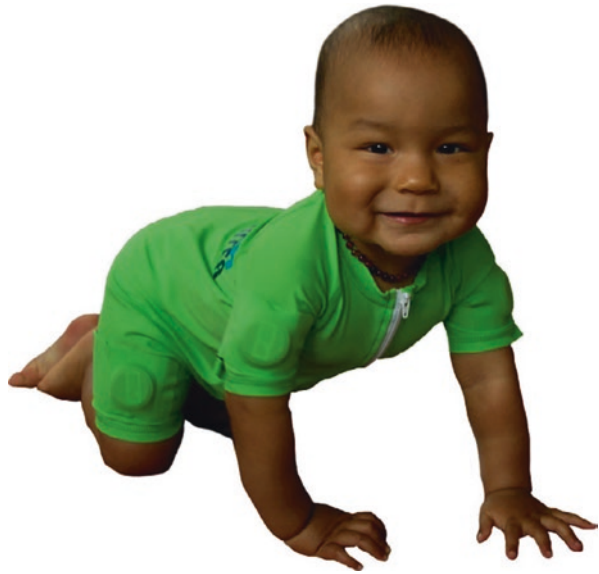
Fig. 2 A 10-month-old subject crawling at home with the MAIJU (Motor ability Assessment of Infants with a Jumpsuit) jumpsuit, equipped with movement sensors in the proximal pockets of each limb. (The image was taken from the open access article in [8])
