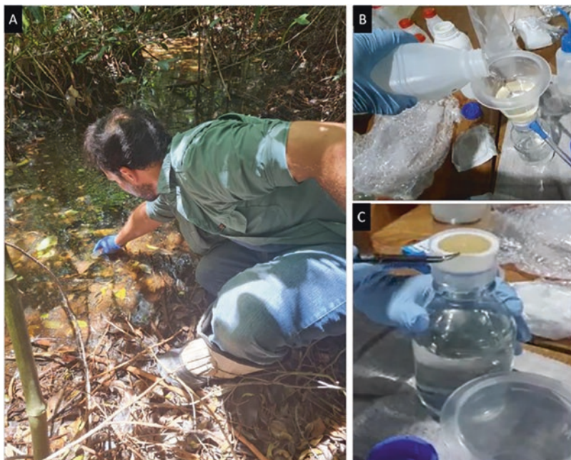
Fig. 18.2 Field and laboratory procedures for water eDNA samples. (a) collection of the water sample; (b) filtration of water samples in a filter using a manual vacuum pump and (c) precipitation of the nucleic acids from eDNA water samples
