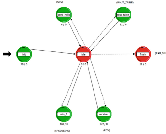
Fig. 5. GEO satellite process model
