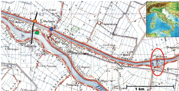
Fig. 1. Map of the investigated area. The orange symbol indicates the position where DFOS and pressure/temperature sensors are installed; the blue one indicates the location the diver for channel water level and temperature monitoring. The red ellipse identifies the downstream dam. The black line represents the section represented in the FE model. The green symbol represents the extracting wells in Adige floodplain.
