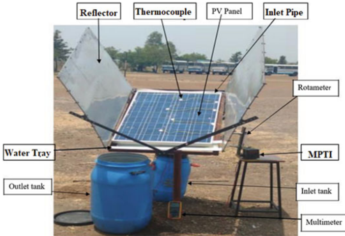
Fig. 3 Conventional photovoltaic system with reflector and with cooling system
