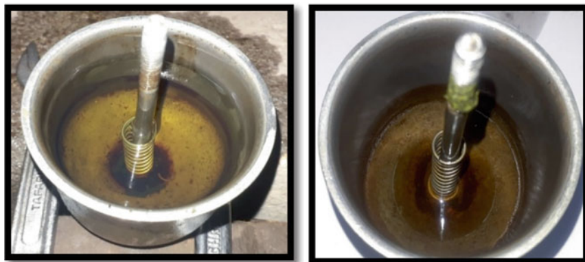
Fig. 7 Condition of fuel filter bottom cup after 100 h test run with a diesel fuel and b WCO biodiesel fuel
