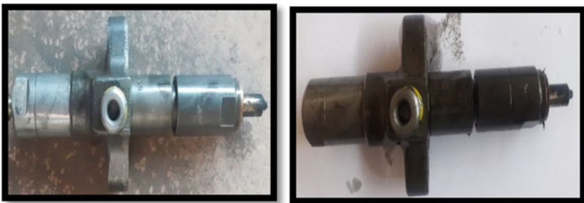
Fig. 2 Injectors condition after 100 h. test run with diesel fuel and with WCO biodiesel
