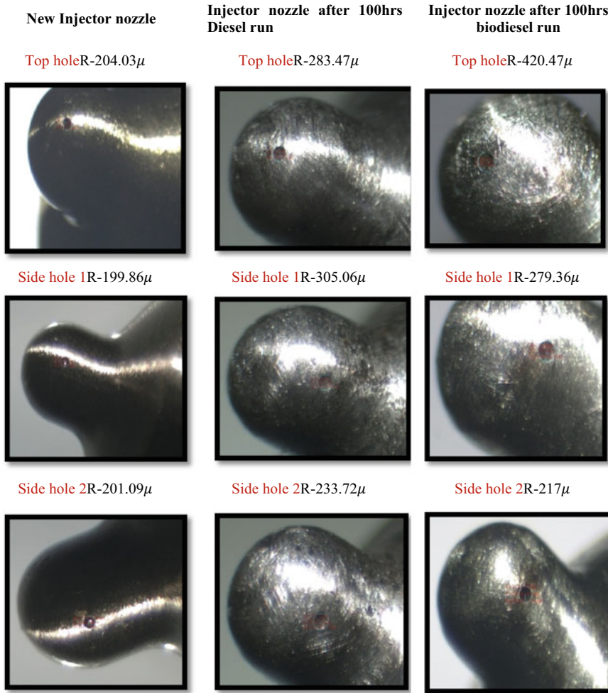
Fig. 6 Nozzle holes radius like top hole, side hole 1, side hole 2 of new injector, 100 h run with diesel and 100 hr run with biodiesel
