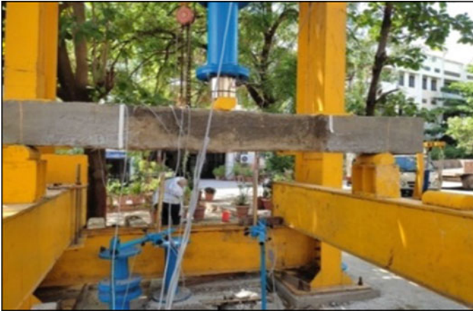
Fig. 7 GFRP jacketing beam test
