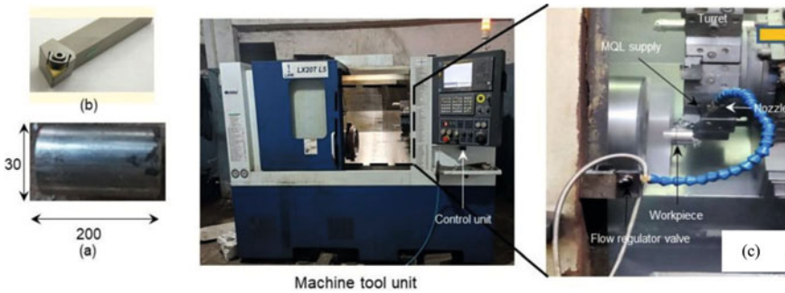
Fig. 1 Pictorial representation of experimental setup a Inconel 718 workpiece, b tool holder, and c enlarged view of experimental setup
