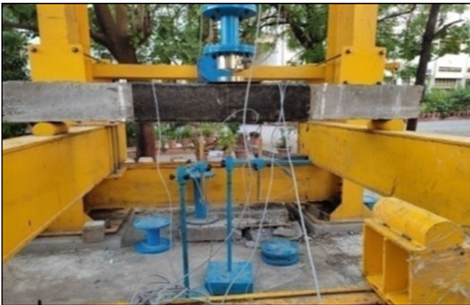
Fig. 8 CFRP jacketing beam test
