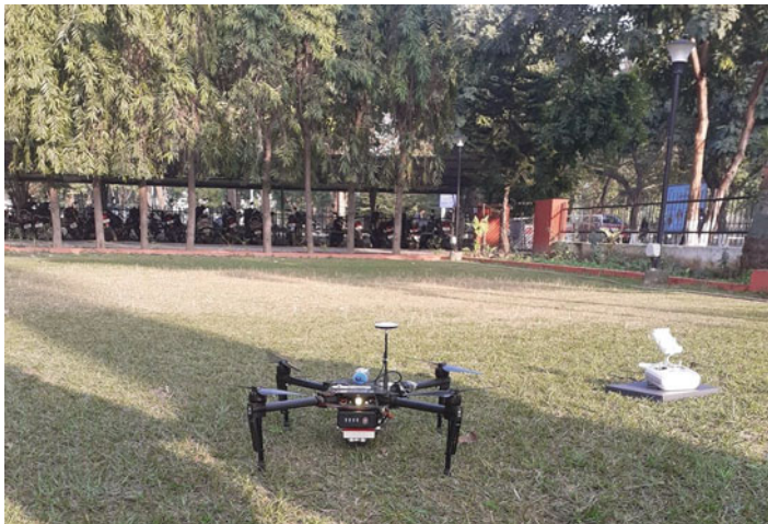
Fig. 3 Unmanned aerial vehicle fitted with a multispectral camera and its controller in white. (Source: Authors)
