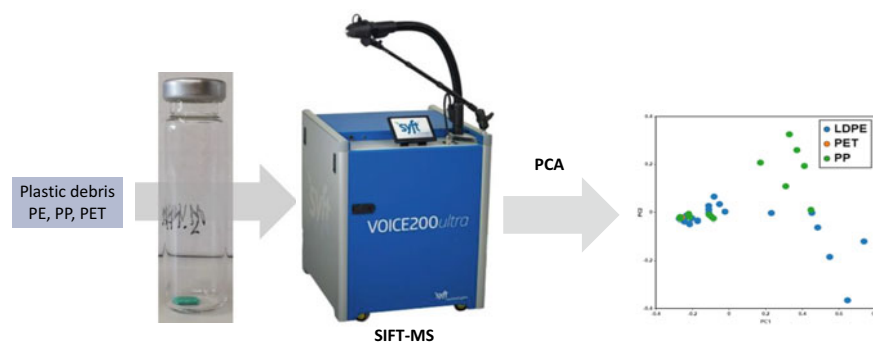
Fig. 8.4 Experimental flowchart for the SIFT-MS analysis of VOCs [9]
