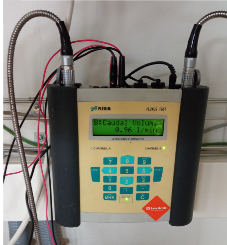
Fig. 3. Portable ultrasonic flow meter
