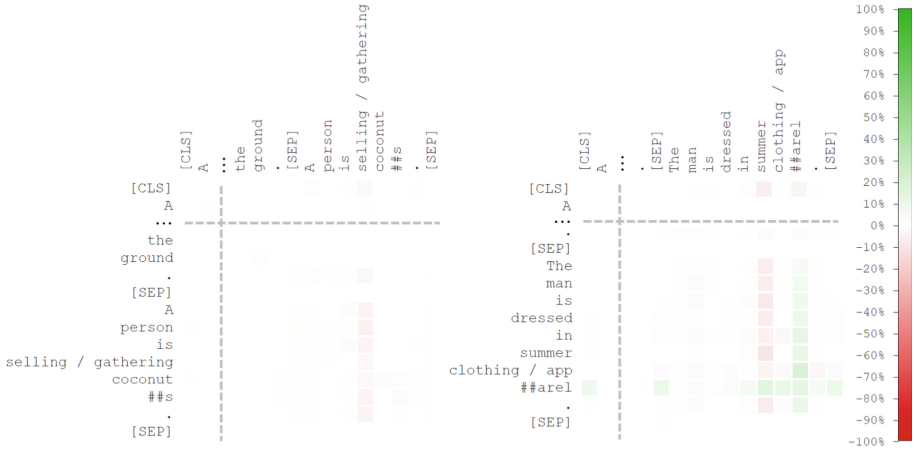
Fig. 3. On the left: Average attention weights difference over all heads for an example adversarial attack with premise “A person wearing a straw hat, standing outside working a steel apparatus with a pile of coconuts on the ground.” and hypotheses “A person is selling coconuts.” and “A person is gathering coconuts.”. On the right: Comparison of the average attention weights difference over all heads for the pair of inputs with premise “A person dressed in white and black winter clothing leaps a narrow, water-filled ditch from one frost-covered field to another, where a female dressed in black coat and pants awaits.” and hypotheses “The man is dressed in summer clothing.” and “The man is dressed in summer apparel.”, respectively. (some irrelevant tokens were omitted to reduce the size of the figure)
