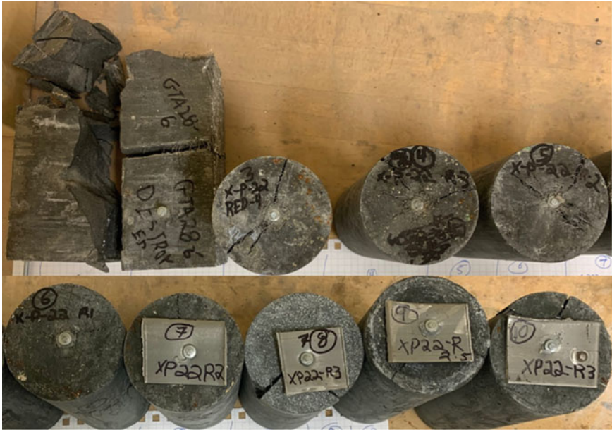
Fig. 7 Images of all the specimens following the penetration tests showing the destroyed and cracked specimens with and without Fe-SMA
