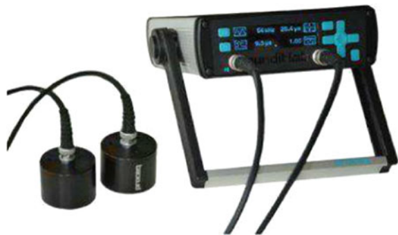
Fig. 2 PUNDIT UPV testing instrument [33]. The pulse velocity can be determined from the following equation:
