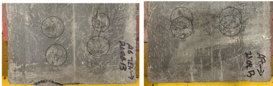
Fig. 8 Side by side images of the CNF-UHPFRC block after the pull-out test A6 (left) and A7 (right). Dotted lines are added to point out the extent of the failure cones
