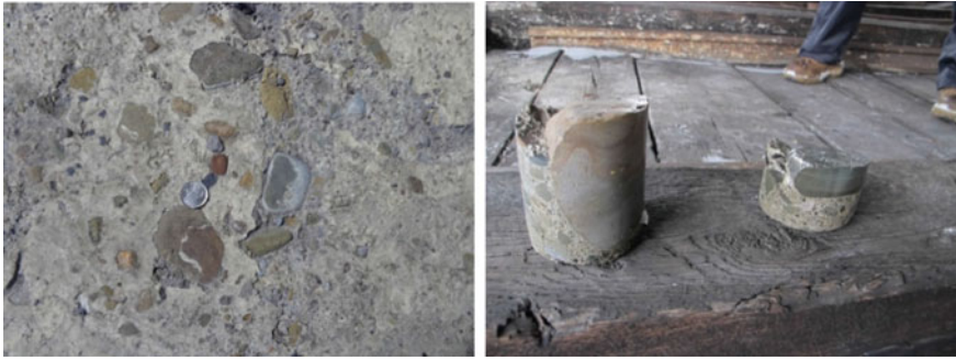
Fig. 11 Views of the surface of the slab at the Greenhill mine tippie building on the left, with a quarter for size, and part of a large stone occupying a large proportion of the area of a 95 mm core on the right
