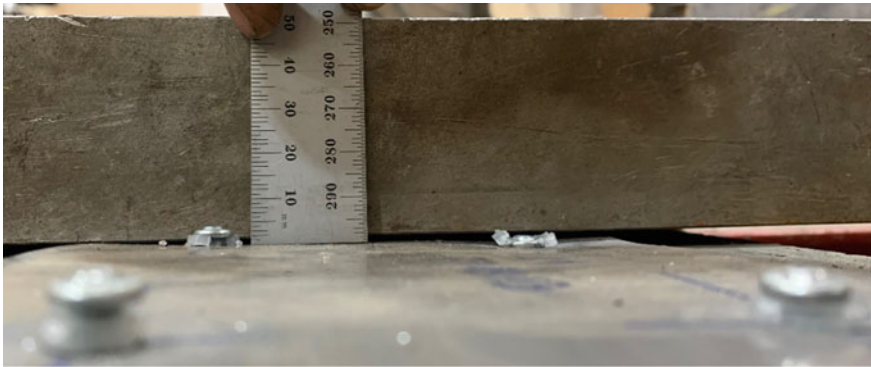
Fig. 10 Surface image of test A9 showing four slightly under-fastened fasteners (27 mm fastener, no pre-drilling)
