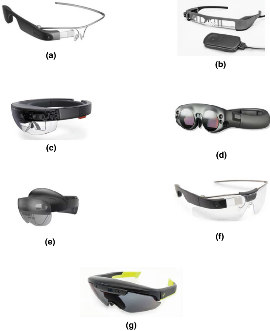
Fig. 2 Typical AR HMDs: a Google Glass Explorer 1, b Epson Movario BT-300 Smart Glass, c Microsoft HoloLens (1st generation), d Magic Leap 1, e Microsoft HoloLens 2, f Google Glass Enterprise Edition, g Eyesight Raptor
