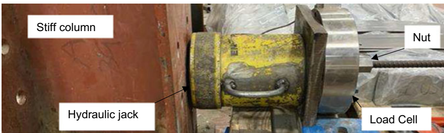
Fig. 4 Hydraulic jack and load cell for recording the force from the pulling system
