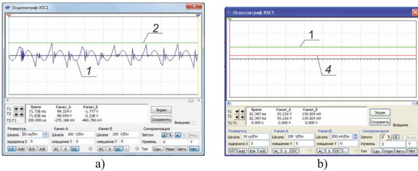
Fig. 8. The results of studies at C1 = 20 \mu\text{F} , wRLS = 75 : a) voltage waveforms on the choke (1) and load (2); b) voltage waveforms (1) and load current (4)
