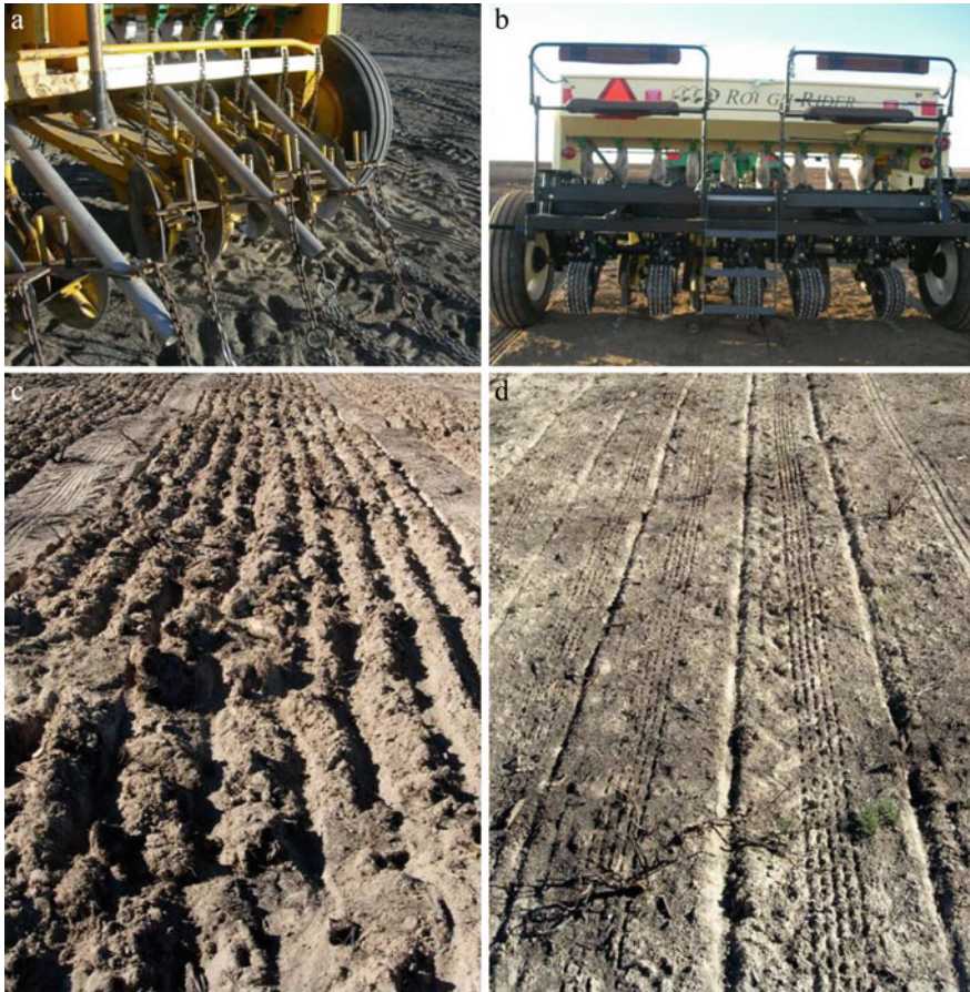
Fig. 5.5 Rangeland drills are designed to seed multiple species at different depths of soil. Traditional rangeland drill (a) that places seeds in furrows (c). In contrast, minimum-till rangeland drill (b) leaves the soil flat (d) after placing seeds. Photo credits. a, b, c and d. Location likely Mountain Home, Idaho in 2006. Photo by US Forest Service. Image currently on Great Basin Fire Science Exchange, Revegetation Equipment Catalog, but originally in Joint Fire Science Final Report, Project #07-1-3-12 by Dr. Nancy Shaw, USFS, https://www.fs.usda.gov/rm/pubs_other/rmrs_2011_shaw_n003.pdf . Photo now found on https://revegetation.greatbasinfirescience.org/wp-content/uploads/2021/01/LRangelandDrillRightMinTillDrill_SoilDisturbance_USFS-294x300.jpg
