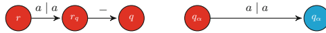
Fig. 4. A transition graph on the left side represents a sub-routine, which replaces each instruction (r, -, q) of \mathcal{M}_R^- , where r \neq q' . The transition graph on the right side represents the transition from \mathcal{M}_R^- to \mathcal{M}_R^+ at the state q_\alpha .
