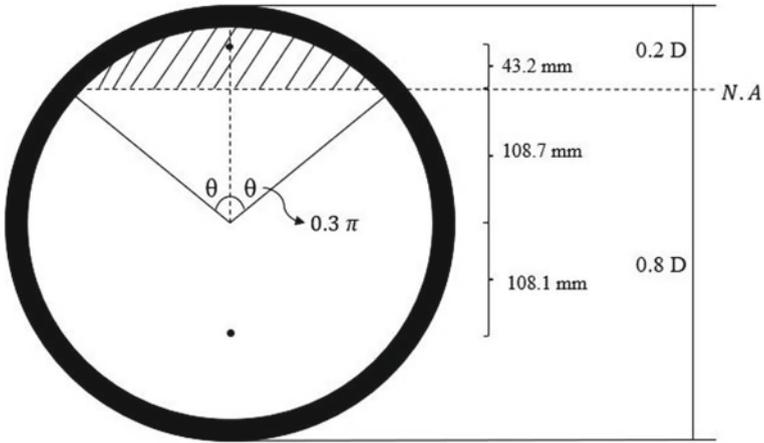
Fig. 4 Cross section of beam when  $c = 0.2 D$
