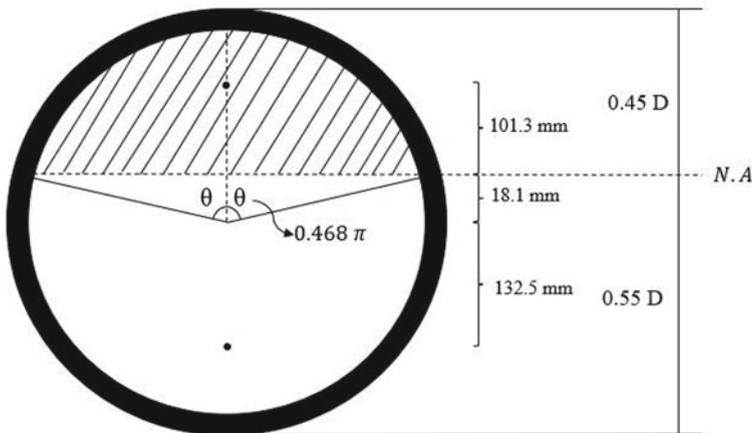
**Fig. 5** Cross section of beam when  $c = 0.45 D$
