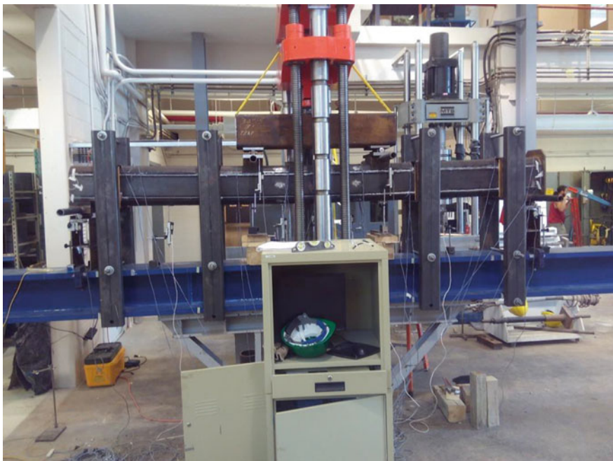
Fig. 5 General view of the four-point bending test setup
