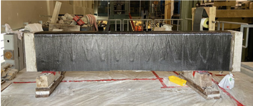
Fig. 2 Beam strengthened with anchored CFRP sheets
