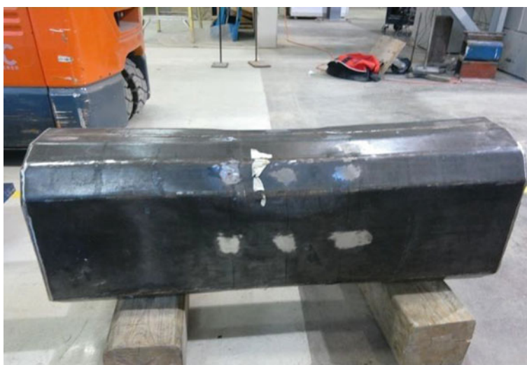
Fig. 18 Deformed shape of the PHS 356 \times 254 \times 6.4 beam
