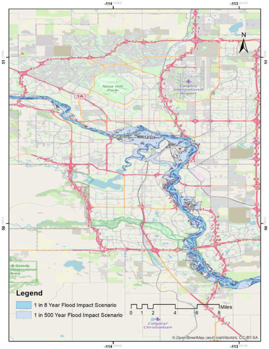
Fig. 4 Spatial representation comparison map of 2013 Calgary flood and a one in eight-year return period flood extent in GIS modelling (Data retrieved from city of Calgary open data portal website [9, 24])
