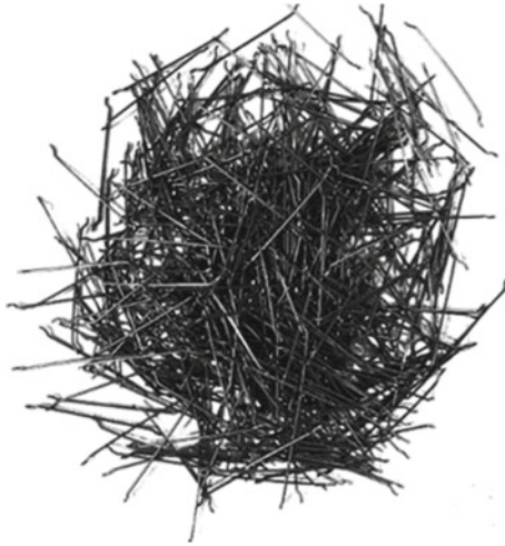
Fig. 2 Steel fibers (type HE-4550)
