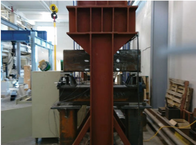
Fig. 15 General view of the three-point bending test setup
