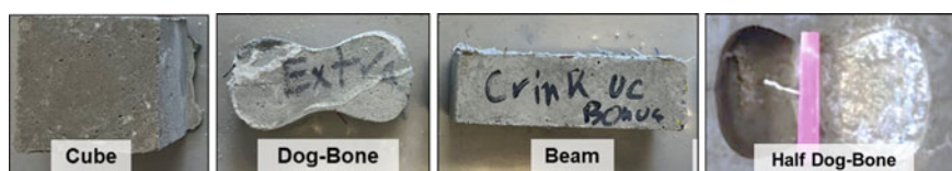
Fig. 4 Illustration for each type of OFPP fiber reinforced mortar sample, viz., cube, dog bone, beam, half dog bone
