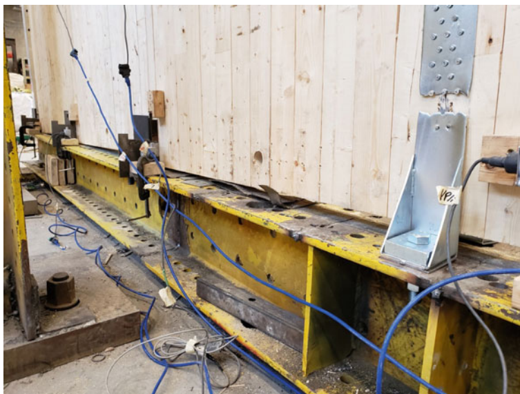
Fig. 12 Lateral behaviour and failure of CLT shearwall experimental test #1
