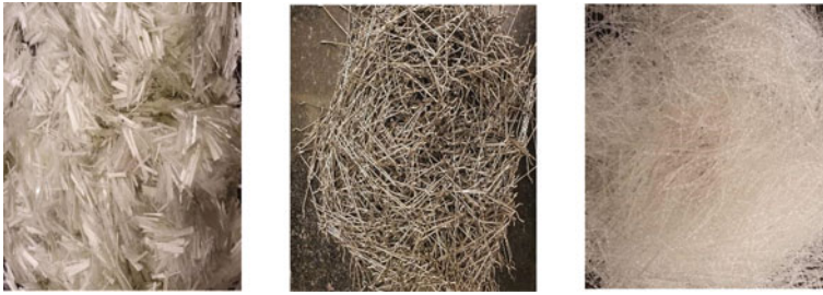
Fig. 1 Sample of the fibers presented with glass fiber, steel fiber, and polypropylene fiber
