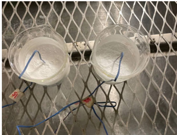
Fig. 4 MPCM 57 inside the environmental chamber attached with thermocouples
