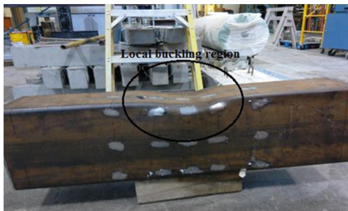
Fig. 17 Deformed shape of the RHS 356 \times 254 \times 6.4 beam
