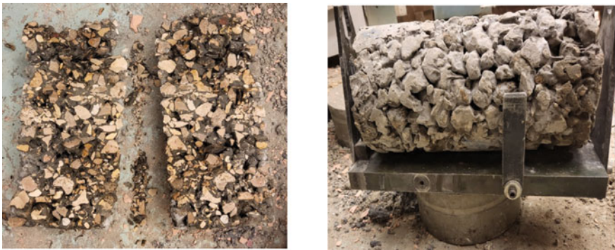
Fig. 7 Examination of splitting tensile test specimen
