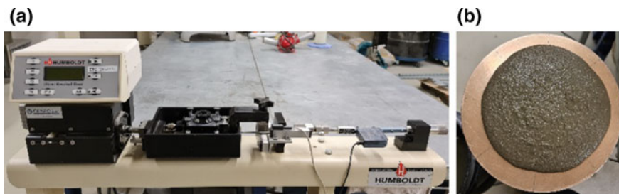
Fig. 2 Modified direct shear apparatus (a) and top view of the flow table (b)
