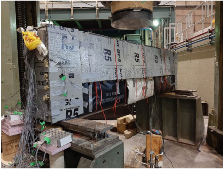
Fig. 6 Power-blankets wrapped on a shear beam for heating before start of test
