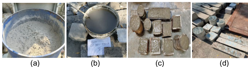
Fig. 2 Mixing of AAC and preparing specimens a dry mixing b solution c specimen d curing
