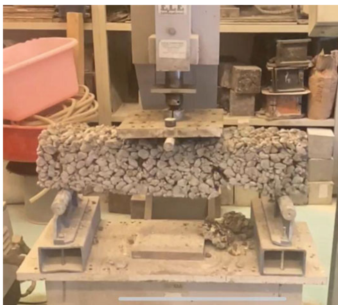
Fig. 5 One-point bending test of pervious concrete beams
