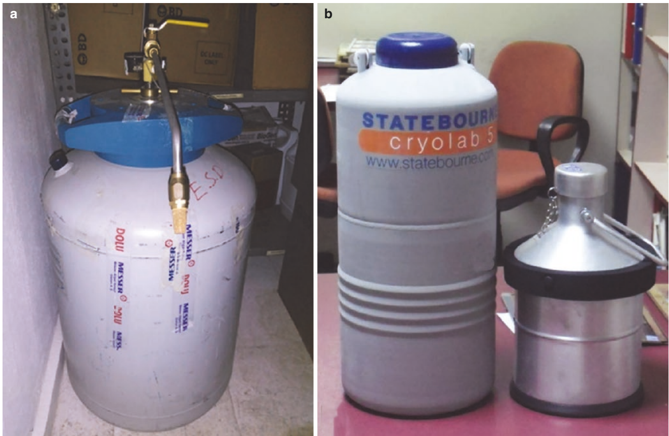
Fig. 5.9 Different liquid nitrogen containers: (a) 60-L capacity, (b) 5-L and 1-L capacity
