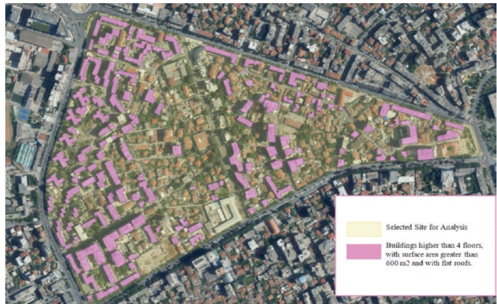
Fig. 1 Selected site and buildings which are suitable for the green roof installation (adopted by author from Google via QGIS)
