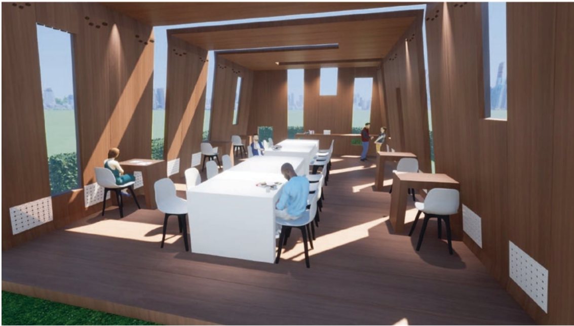
Fig. 17 Inner face of the multi-regulation bio-envelope integrated into the pavilion. It shows the inner side of the “air pumping mechanisms” in the lower part of the envelope, besides the chimney holes in the upper part of the envelope
