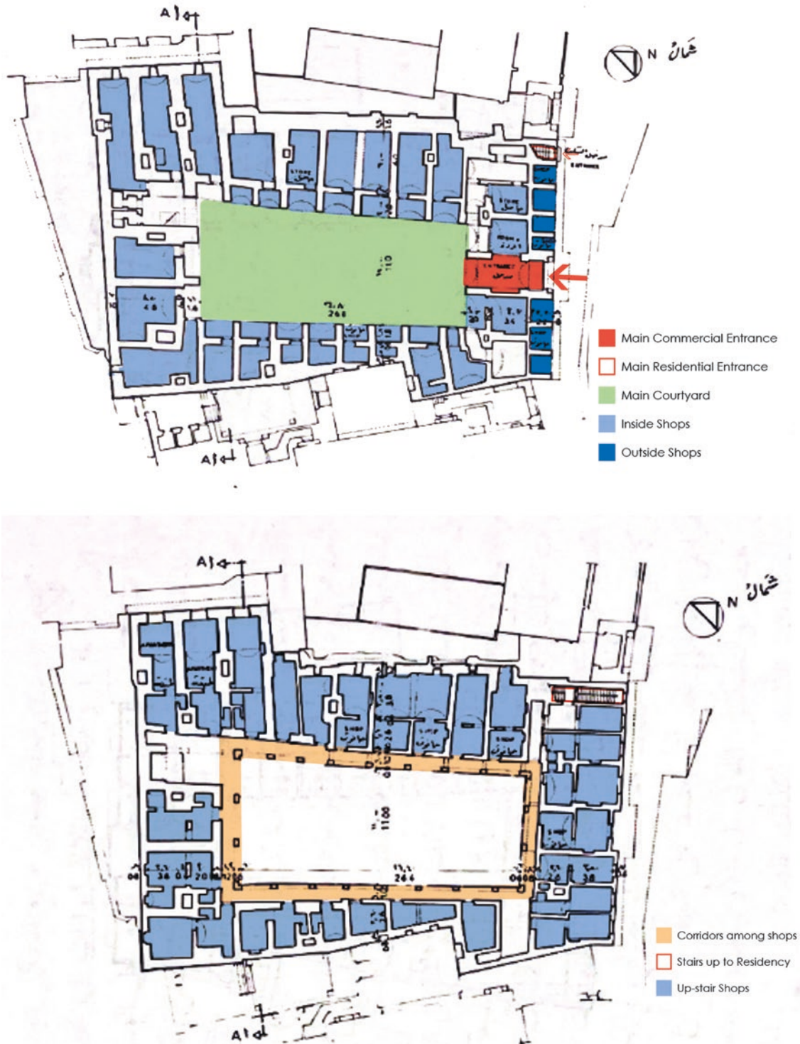
Fig. 21 Zoning of both a ground floor plan and b first-floor plan. Source The Organization of Islamic Capitals and Cities (OICC), edited by the researcher
