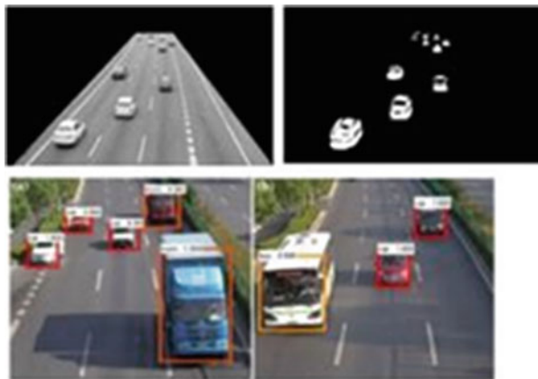
Fig. 8 Vehicle extraction using a deep neural net [9–12]
