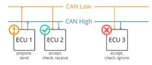
Fig. 3 ECU communication through CAN bus [21]
