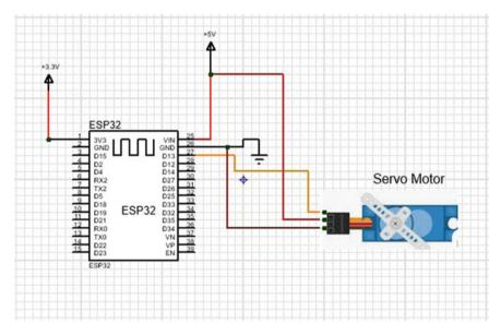
Fig. 15 The connection of the servo motor to the ESP32 MCU
