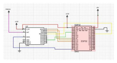
Fig. 14 Connection of the LoRa transceiver to the ESP32 MCU
