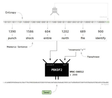
Fig. 17 Operation diagram of BIP39 [18]
