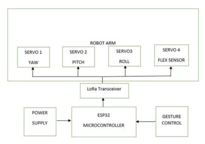
Fig. 31 Block diagram of the microelectronic unit and the servo motors embedded in the robotic arm
