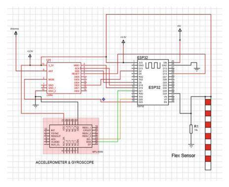
Fig. 20 Circuit diagram of the transmitter for the gesture control of robotic arm via LoRa technology
