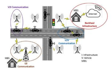
Fig. 1 CAV basic system architecture [16]
