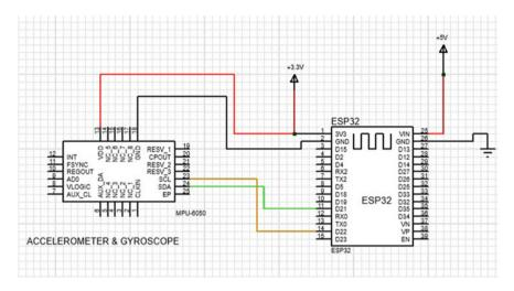
Fig. 13 Connection of the accelerometer and gyroscope to the ESP32 MCU
