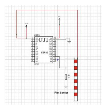
Fig. 12 Connection of the flex sensor to the ESP32 MCU
