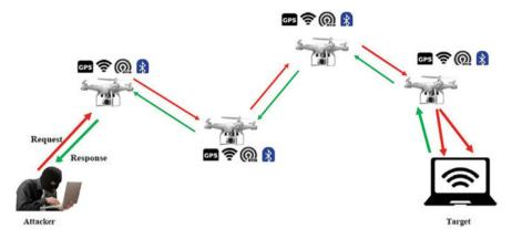
Fig. 4 Stepping stone attack using multiple UAVs
