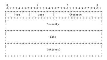
**Fig. 10** Secure RPL control message as shown in [53]. The ICMPv6 information message with a type of 155. The code identifies the type of the RPL control messages (DIO, DAO, DIS, etc.), and the checksum computation field that is computed for each security message
