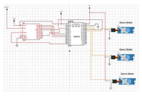
Fig. 21 Circuit diagram of the receiver of the gesture control of robotic arm via LoRa technology
