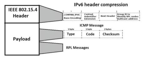
Fig. 5 IEEE 802.15.4 frame with the header and the payload sizes as defined by the 802.15.4 specifications
