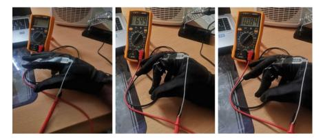
Fig. 27 Flex sensor resistivity on multimeter
