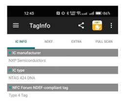
Fig. 31 NFC tag information scanned via NPC's TagInfo application from Android phone
