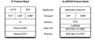
**Fig. 4** IP and 6LoWPAN protocol stacks as presented in 6LoWPAN the wireless embedded Internet by Shelby and Bormann [45]. The representation of each layer in the 6LoWPAN shows how the logical communication between the layers at the same level can be interpreted, i.e. communication between the IP network layer and IPv6
