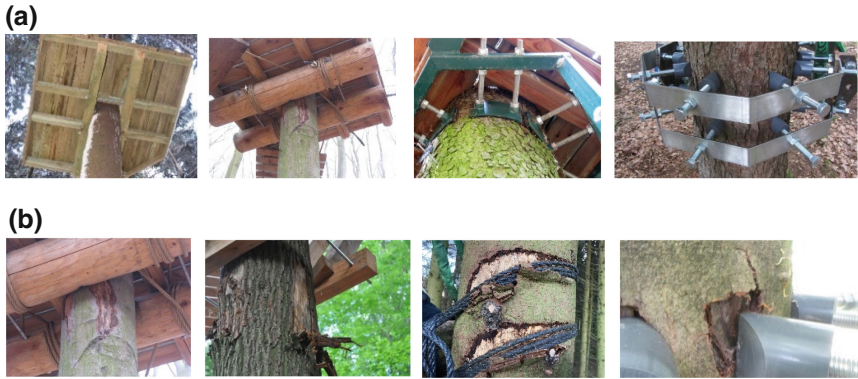
Fig. 4. a) Examples of different methods of friction-based force transfer b) Failure mechanism of a friction-based force transfer.
