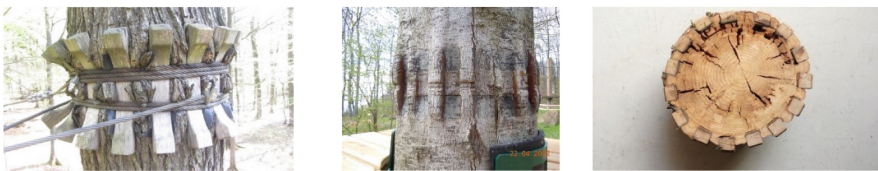
Fig. 3. a) Form-locking force transfer through the stems surface using wrapping techniques. b) Different grades of failure under usage of wrapping techniques.
