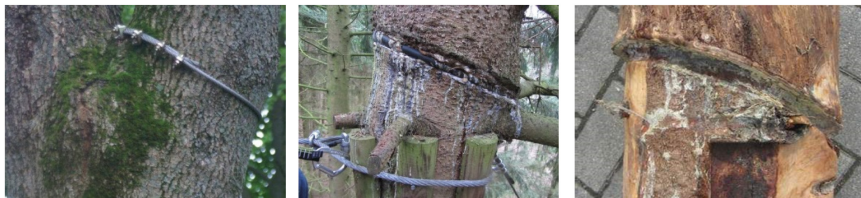
Fig. 2. a) Form-locking force transfer through the stems surface under usage of textile slings. b) Result of form-locking force transfer under usage of textile slings when contact stress is greater than the cambium growth pressure. c) Result of form-locking force transfer under usage of (covered) steel cables when contact stress is greater than the cambium growth pressure.
