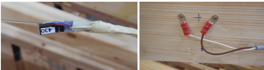
Fig. 1. Left: relative humidity sensor and thermocouple/Right: wood humidity sensors.
